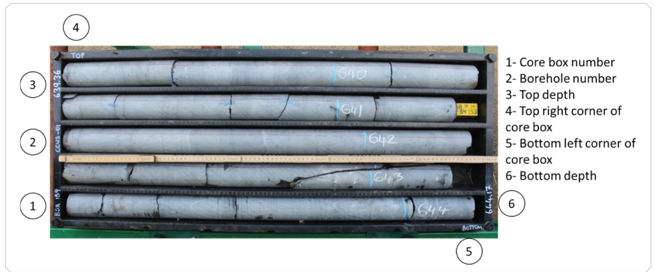
Figure 1: NQ core tray with core of the dolomite successions starting from a 639.39 m to 644.17 m. The numbered annotations indicated various labels on the core trays.
