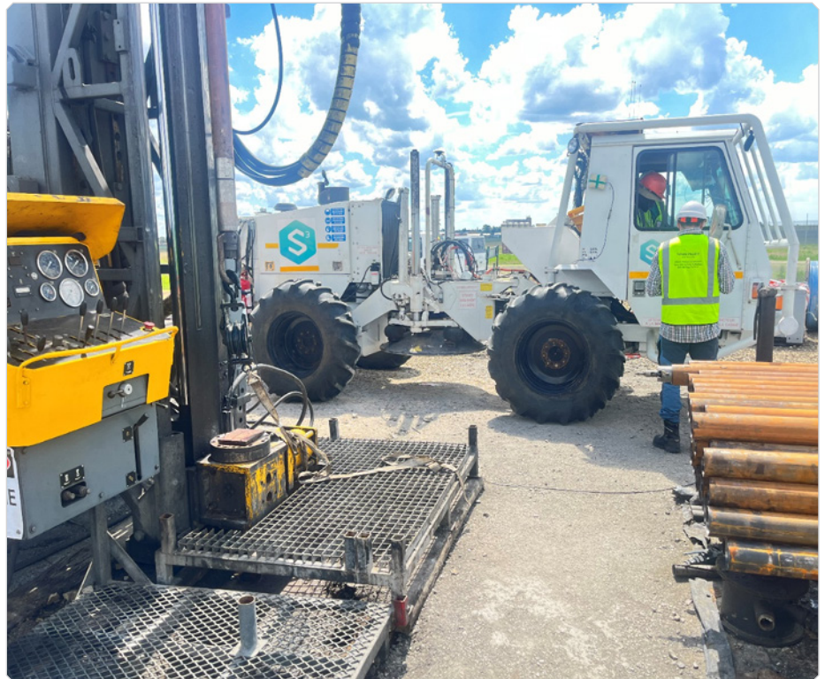
Figure 3: Vertical Seismic Profile (VSP) data acquisition using optic fibre and an 8-ton mini vibroseis truck as seismic source.
