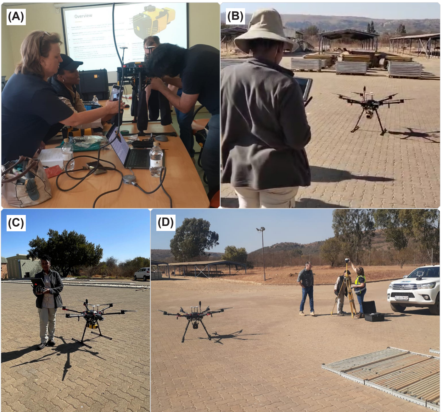
Figure 3. Preparation for data collection a) and c) Mounting the YellowScan LIDAR sensor, b) Pilot-in-Command ready for take-off and data collection d) GPS base and rover ground control points.
