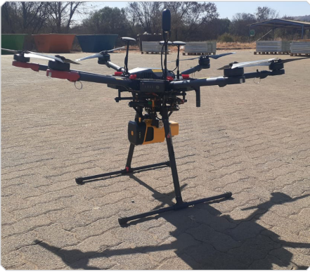
Figure 2. Matrice 600 pro mounted with the YellowScan LIDAR sensor.
